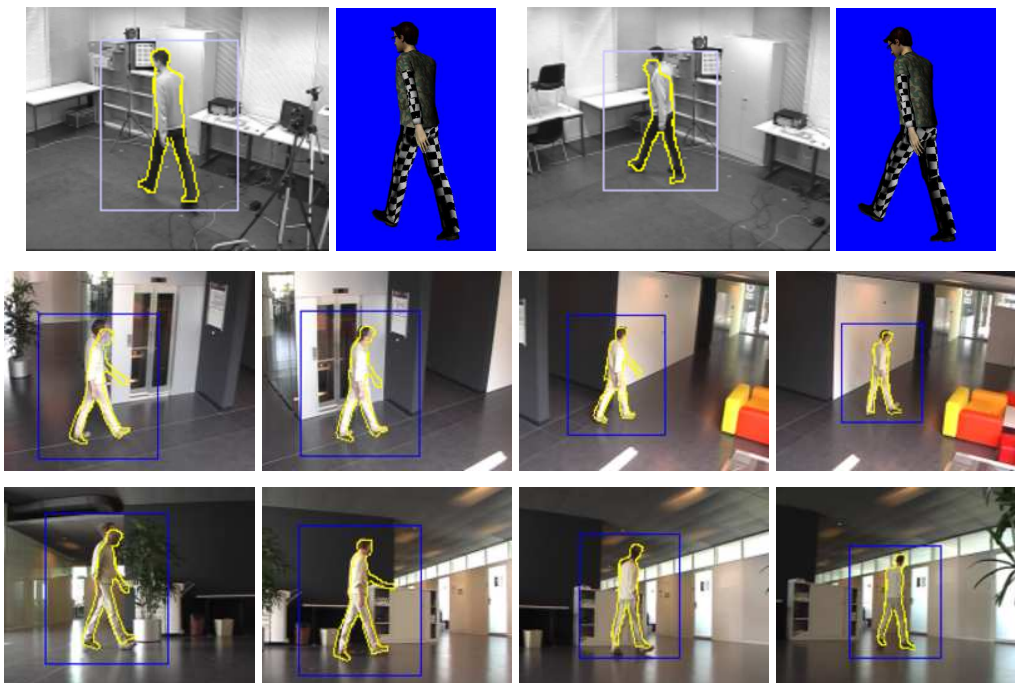
Fig. 10. Robustness to changes in camera height. First two rows: The 3-D pose is correctly recovered even though the actual camera is much further above ground level than the virtual cameras used to create the templates. Third row: Correctly detected silhouettes when the camera is placed only 30 cm above the ground level.
