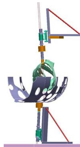
Port assembly support; can be moved in all directions. The ports will be positioned between the inner and outer openings with the help of a movable sledge.
