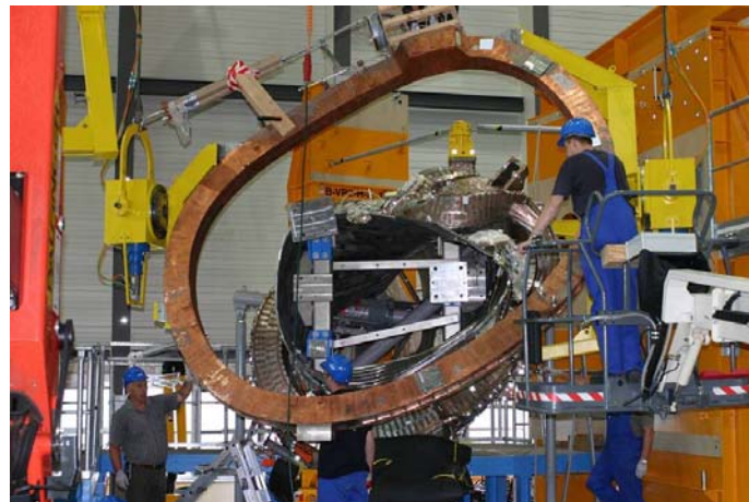
Design and procurement of different coil stringing tools and mounting stands
