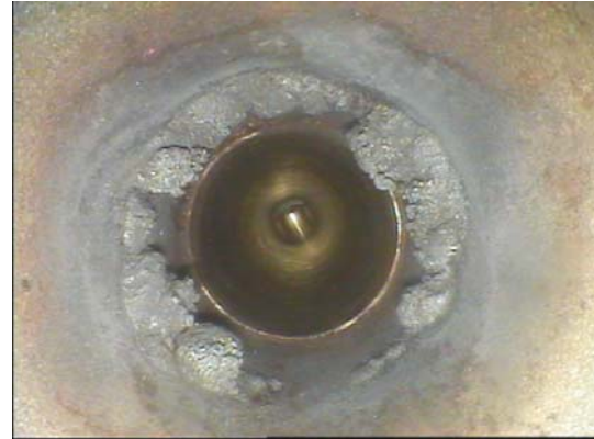
Thickness measurement of the winding package insulation of non planar coils
