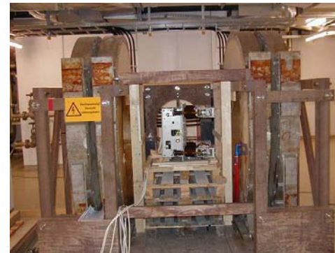
Test of a circuit breaker in the magnetic field (test bed in Greifswald) 51
