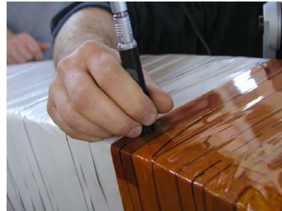
Thickness measurement of the winding package insulation of non planar coils
