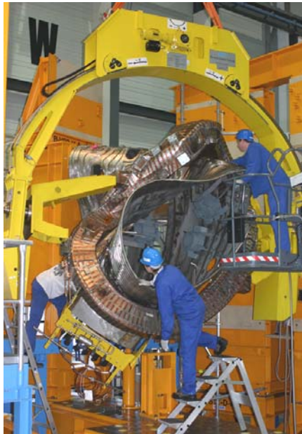
Design and procurement of different coil stringing tools and mounting stands
