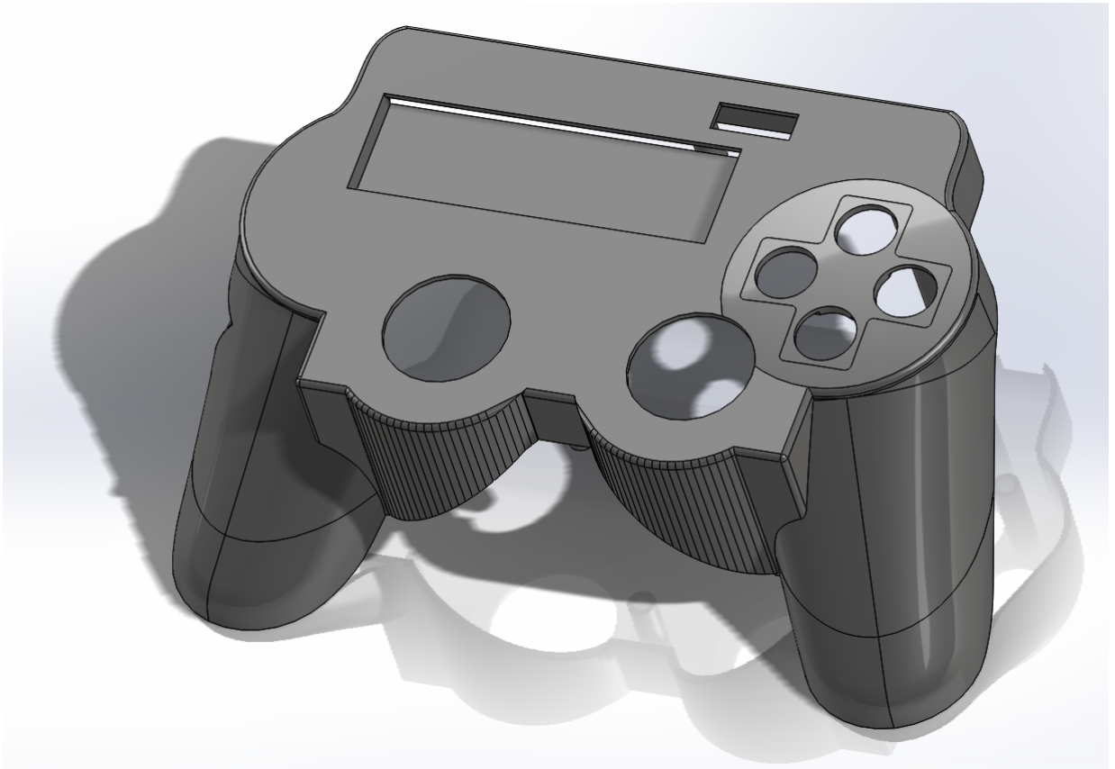
Figure 6.3: Top view of theSolidWorks 3D model of the top part of the remote control
