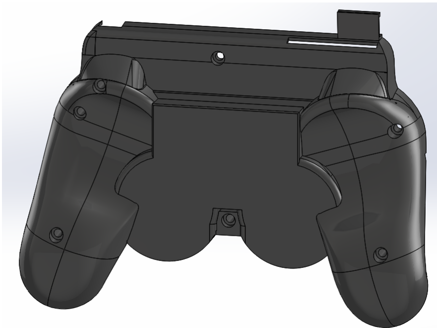
Figure 6.6: Bottom view of the SolidWorks 3D model of the bottom part of the remote control
