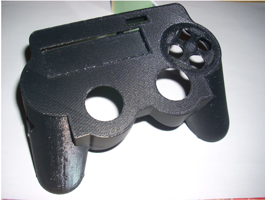
Figure 4.2: Top part of the 3D printed remote control
