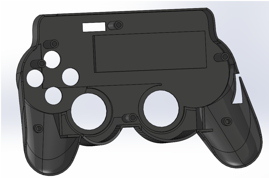
Figure 6.4: Bottom view of theSolidWorks 3D model of the top part of the remote control
