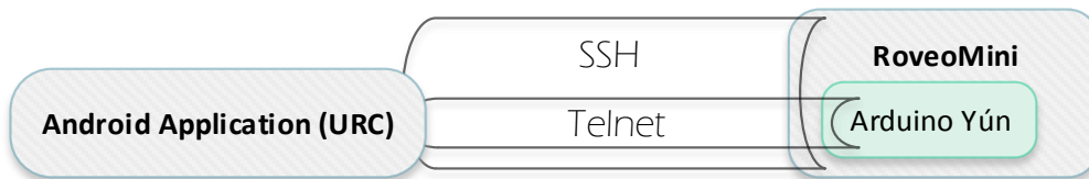
Figure 2.10 – Communication schema of the ROVéo Mini with the URC.
