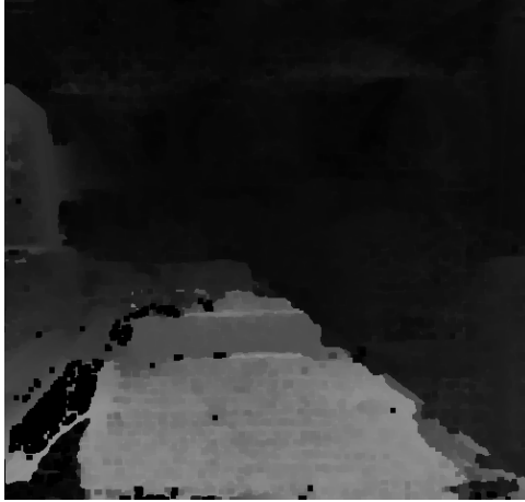
Figure 17: Depth map after closing with a kernel size of 9
