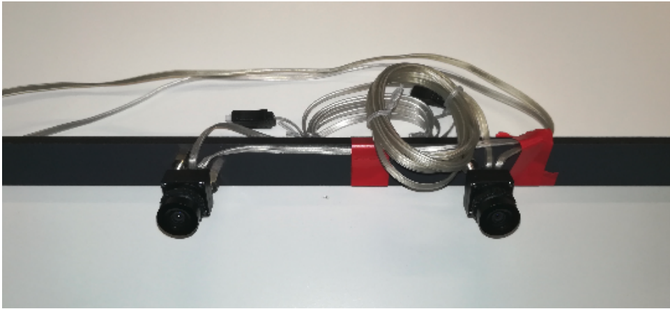
Figure 2: Stereo camera using two Ximea cameras
