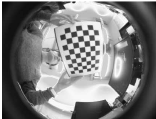
Figure 13: Sample image for calibration with the checkerboard
