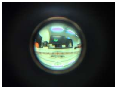
(a) Fisheye lens with a focal length of 1.05 mm which was originally intended to be used for EnVision
