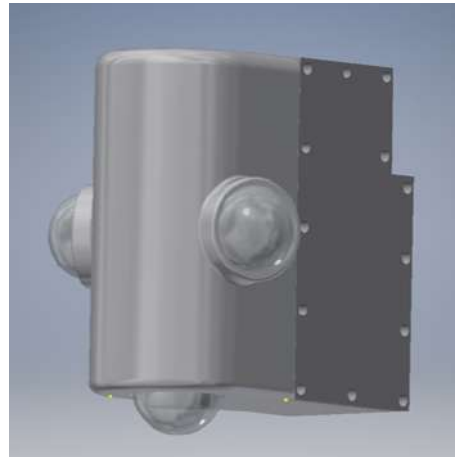
(b) CAD model of the assembled head unit including eye domes and lid
