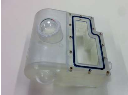
(a) Head module after assembly of thread inserts, rubber tube and glass domes
