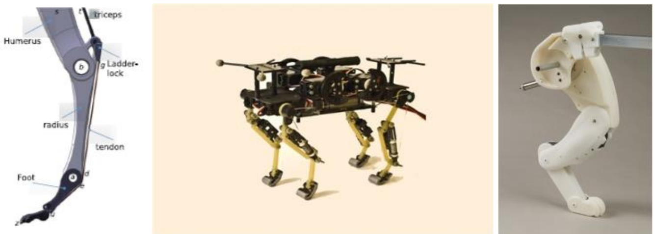
Figure 1. Some feet implementation in quadruped robots. Left: MIT Cheetah robot Middle: Cheetah-Cub BioRob Robot Right: HRL Laboratories
