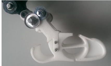
Figure 10 Locked Tarsal-Metatarsal joint in -15^\circ position. The screw behind the moving axis (star-locker) blocks the joint movement.
