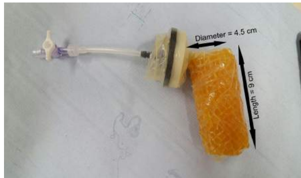
Figure 7: The variable stiffness element we designed and used to retrieve our medium's Young's modulus, in its vacuumed state. The membrane has been shaped with the hard shell beforehand. An airtight switch in the off state is attached to the base, ensuring the airtightness of the element when removed from the pump. The diameter is 4.5 cm and the length 9 cm.
