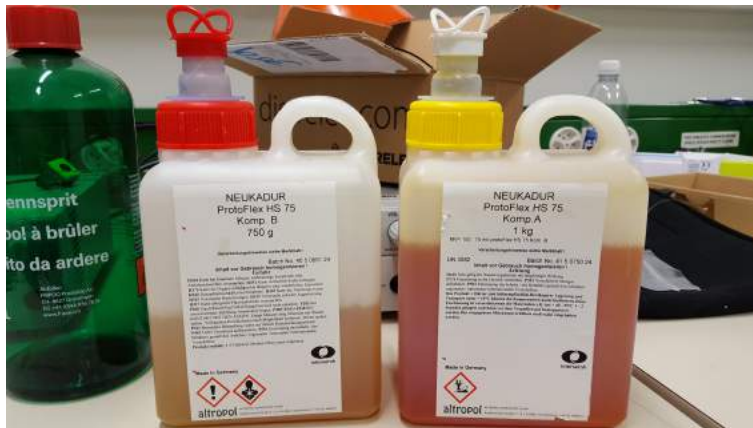
Figure 2: The two components Neukadur ProtoFlex HS 75A polyurethane elastomer from Altropol used to create the granules.
