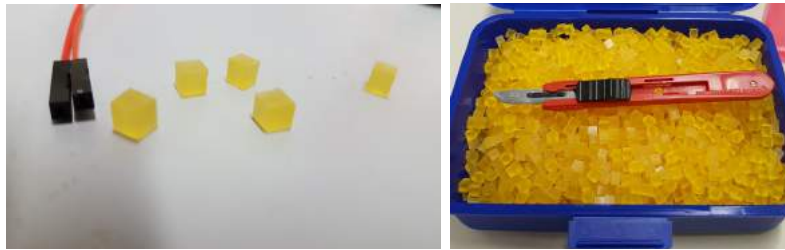
Figure 4: LEFT: 4x4x4 mm cubes elastomer cubes used as medium. RIGHT: Total amount of cubes retrieved and the scalpel used to cut them.
