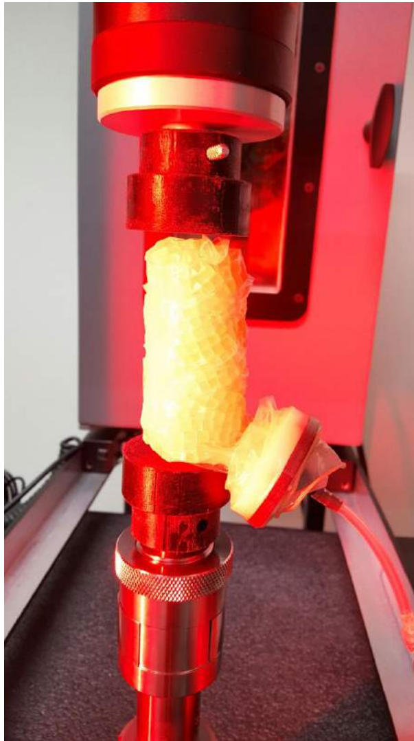
Figure 11: A view of the element ( specimen ) between the force transmitters of the extensometer. The red light comes from the extensometer's video module and enhances the contrast in order to further evaluate the lateral expansion of the specimen (NB: we did not use this feature for our experiments). One can easily see that the base is tilted to the side in order for it not to get in the way of the load transmitters.
