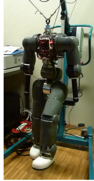
Figure 7.6: Configuration of the real CoMan (hung by real ropes) when the stimulation has reached its higher value (1.0).
