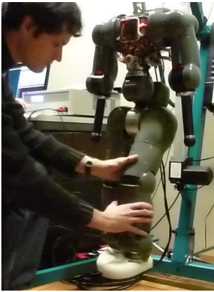
Figure 7.13: Interaction on the left leg while the HFL virtual muscle has a maximal stimulation
