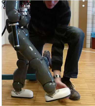
Figure 7.30: Reflexes test on the right leg - current time: t = 30.7 s
