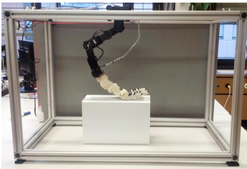
Figure 4.1: Experimental montage that comprehends a robotic 2 DoF leg and a supporting structure.
