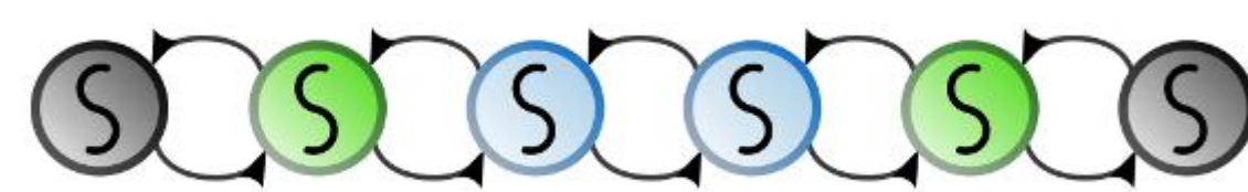
Figure 2. The corresponding (to 6 motors) Central Pattern Generator (CPG) neural network . CPG is a simple, but flexible parameterized movement model. It was discovered in the neuroethology that CPG serves many functions in vertebrate animals.
