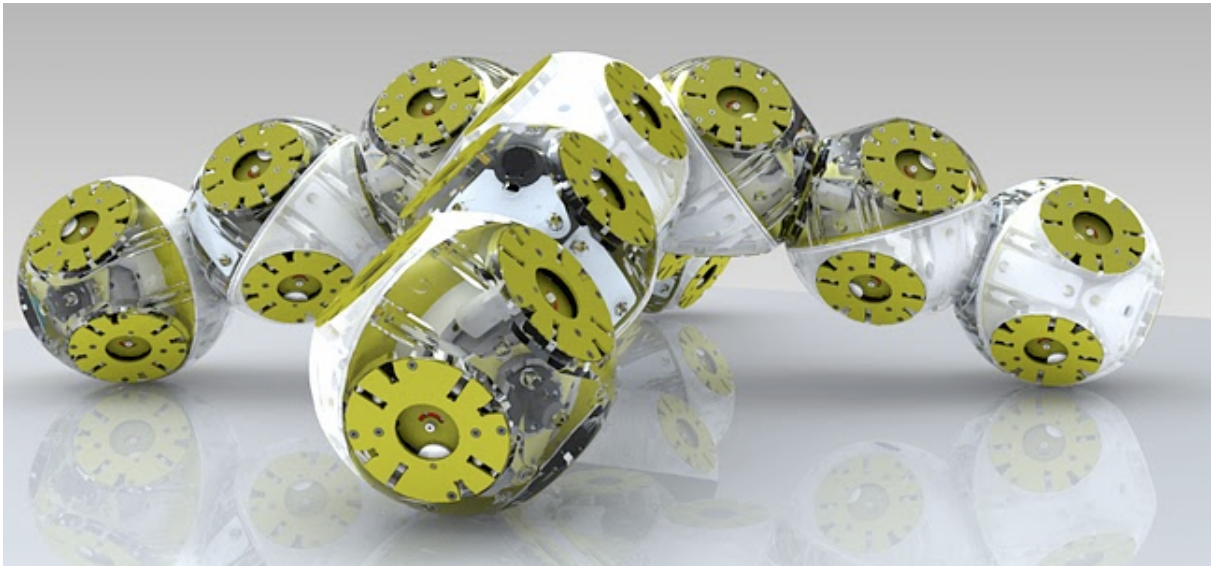
Figure 1.3: Roombot modules. Image from BIRG [4]
