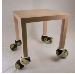
Figure 9: Four Roombots modules connected the Lack ikea table [20, 27].
