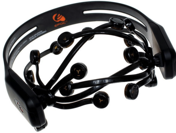
Figure 5: Emotiv EPOC from Emotiv Systems. It possess 14 EEG channels. Its sensor technology relies on saline soaked felt pads that have to be prepared before each use. The sample rate is 2048 [Hz], filtered and downsampled to 128 [Hz]. It also possesses a 2-axis gyroscope [3].
