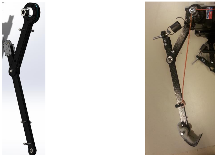
Figure 11: Leg design (on the left) and final product (on the right)
