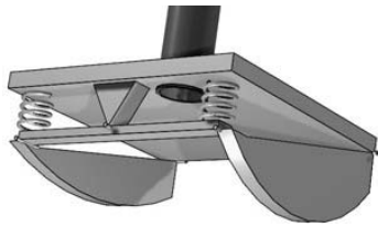
(a) Schematic diagram of the foot of the walker [HWR01]
