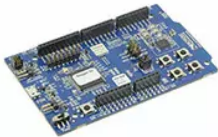
Figure 4: The Nordic nRF51 development kit used in the system implementation.
