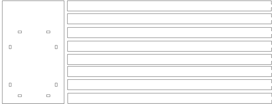
Figure 11: Parts to cut from MDF, the size of the plate used is 400x150 mm.
