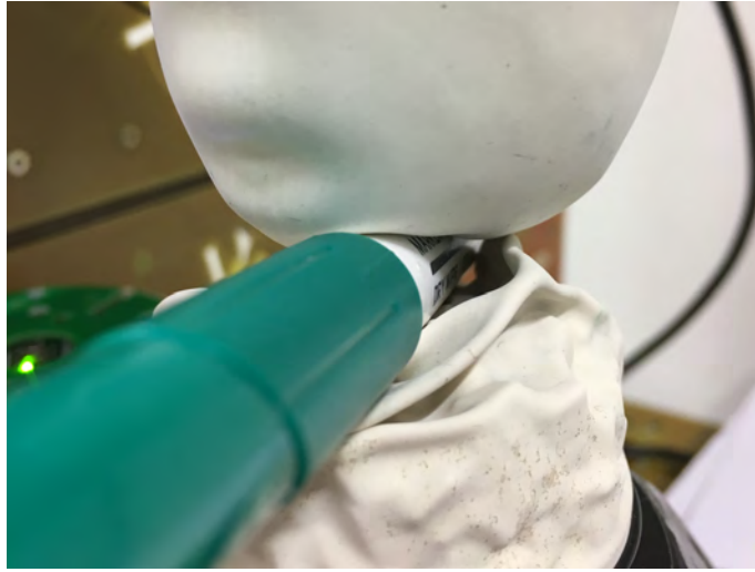
Figure 18: Resulting membrane aspect once the object has been released from the gripper
