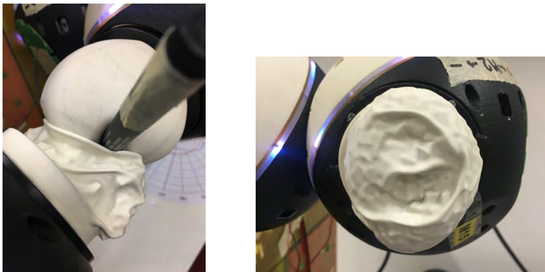
(a) Intermingling of membranes during passing motion (b) Resulting gripped shape. The circular fold caused by the first gripper clearly visible.
