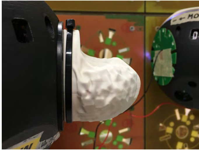
Figure 17: Asymmetry of the receiving gripper (vacuumed) caused by the gravity
