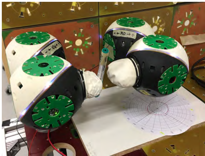
Figure 1: Successful sideways passing of a pen between two Roombots modules
