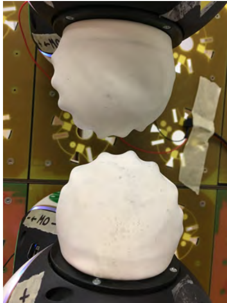
Figure 14: Corrugated profiles of membranes when not fully inflated
