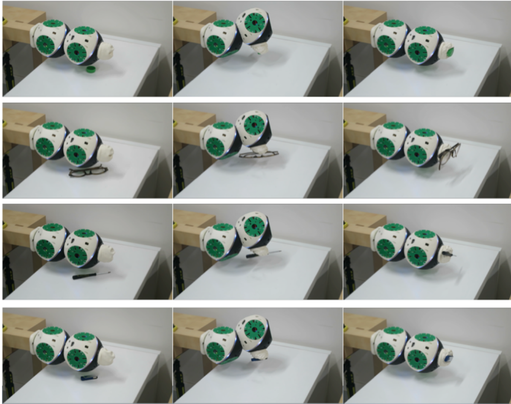
Figure 16: Various object pick up: bottle cap, glasses, screwdriver and USB key
