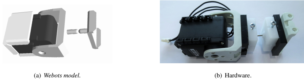
Figure 3.3: Module composed by Dynamixel motor, lever arm and passive element.
