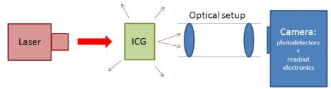
The laser used excites ICG molecules which then emit fluorescence photons. The optical setup permits to carry a maximum of these photons to the camera.
