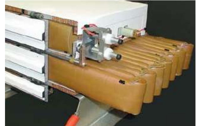
Northrop Grumman Astro Aerospace Flattenable Foldable Tubes for the Mars Express (Adams et al., 2009)
