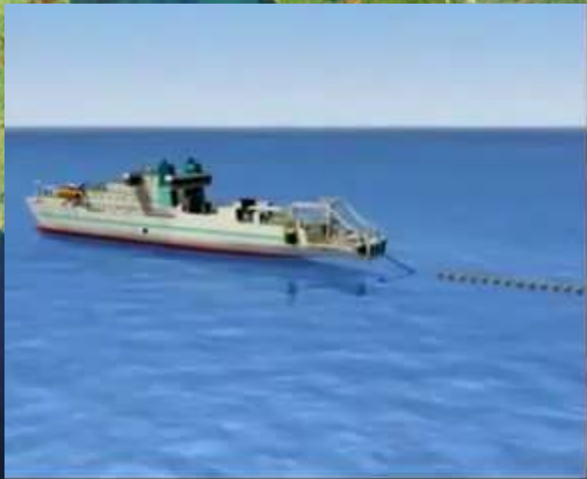
Submarine Cable Deployment Global Marine Systems
