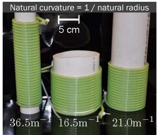
Curvature induced by wrapping around cylinders
