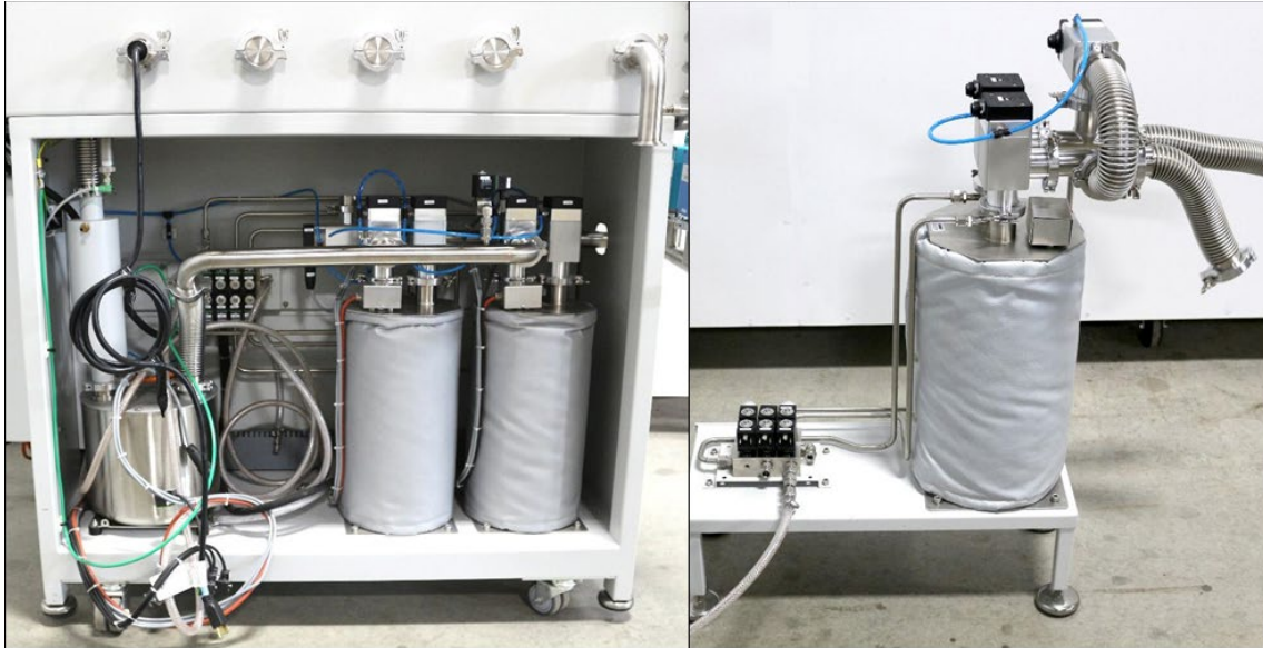
Figure 8: Left: Example of a purifier system with two separated canisters. These canisters can be duplicates, each containing a mixture of molecular sieve and copper catalyst OR the first canister contains the molecular sieve or the activated carbon and the second one contains the copper catalyst. Right: Example of a purifier system with only one canister containing a mix of molecular sieve and copper catalyst.
