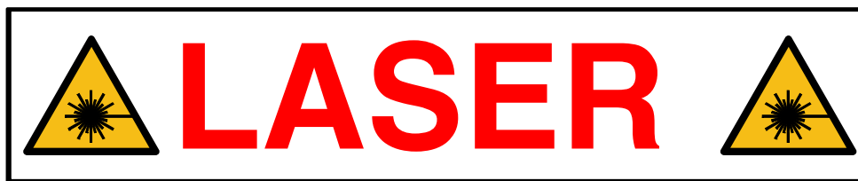
Figure 5 Laser warning panel. White background, red letters and ISO 7010 warning sign.
