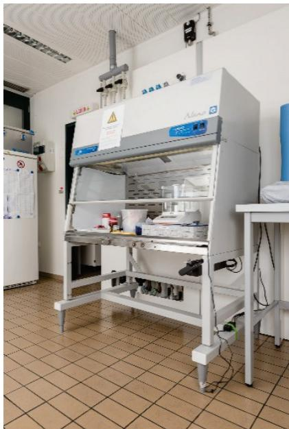
Similarly to a nano enclosure, a biosafety cabinet has a controlled air flow that allows for work with pathogens safely. The controlled air flow is extracted from the inside of the hood, and is filtered before being released in the atmosphere. Biosafety cabinets can provide some protection when handling ENM, if an adapted filter is used.
