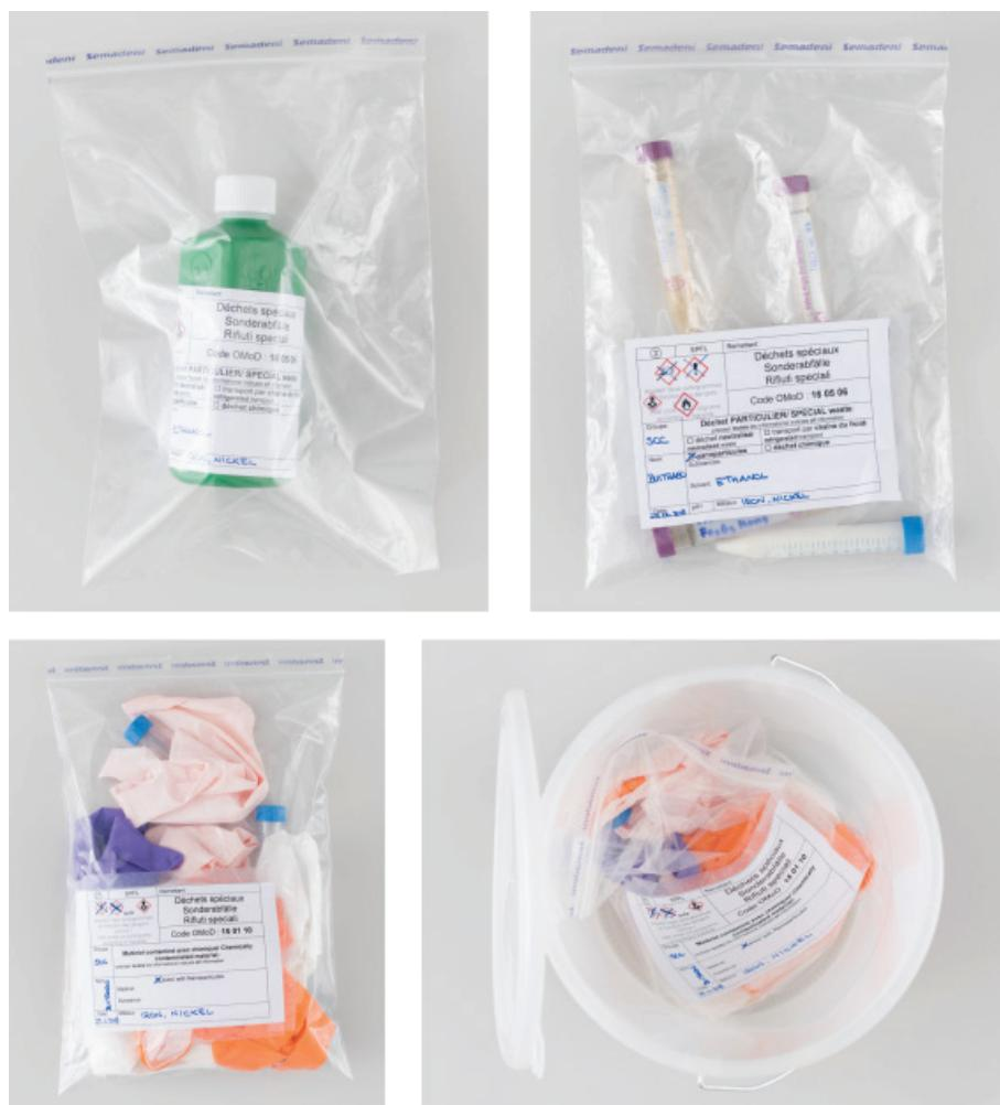
Figure 6: Double packaging of nanomaterial waste.
