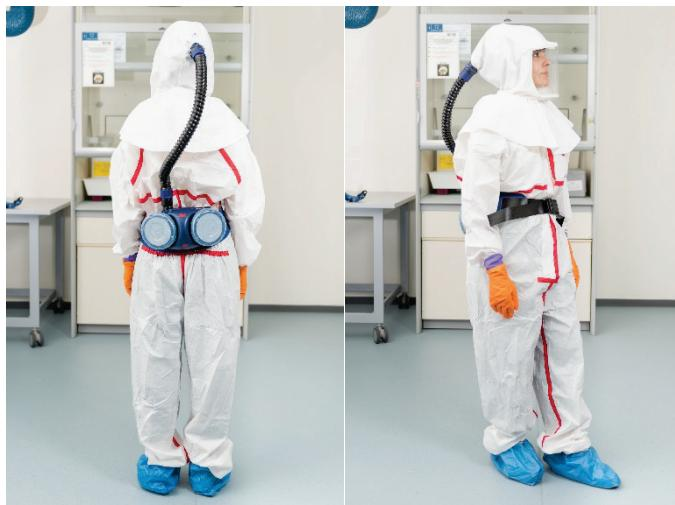
Figure 4: Personal protective equipment for work in a Nano 3 lab.
