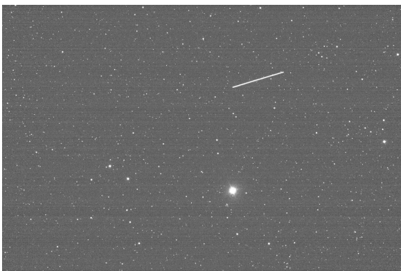
Figure 3: Example of a satellite track. In this image, the satellite in question is a Starlink satellite from the company SpaceX. The exposure time is 0.5 s.
