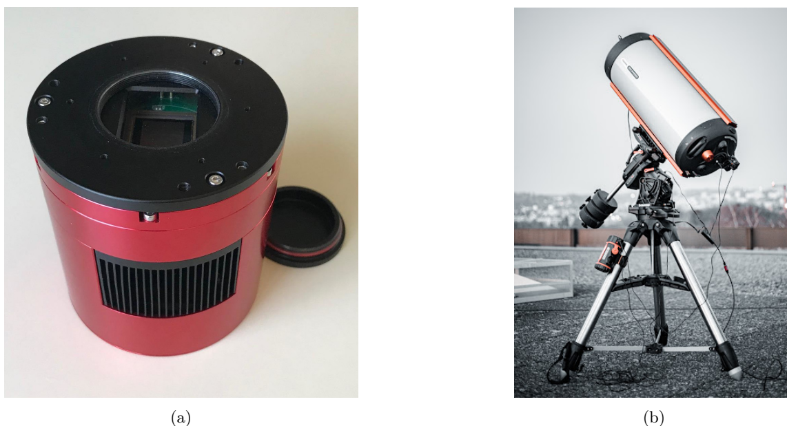
Figure 6: a) ZWO Mono astrocamera used for observations b) Telescope and mount image by Yan Crevoisier.
