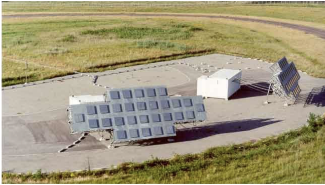
Fig. 2. Emission site for the GRAVES system. There are 4 panels containing 28 patch antennas each.
