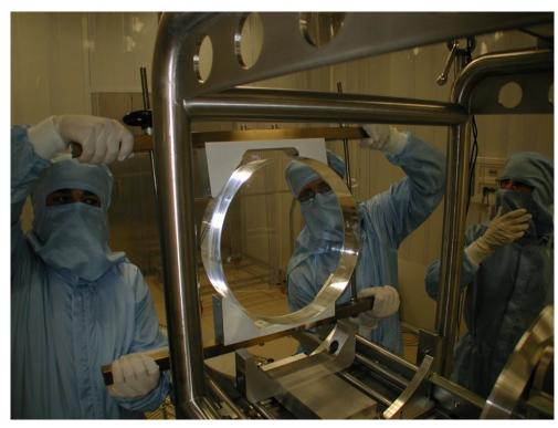
Coating of mirror surfaces performed at LMA (Laboratoire des Matériaux Avancés) in Lyon
