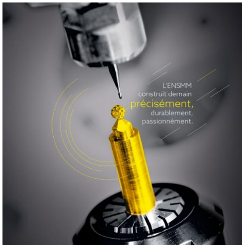
The smallest micromanufactured soccer ball in the world (32 parts) S. Thibaud – ENSMM - 2019
