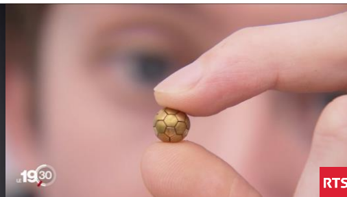
The smallest micromanufactured soccer ball in the world (32 parts) S. Thibaud – ENSMM - 2019
