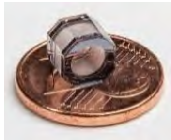
Atomic clock with microfabricated cell
