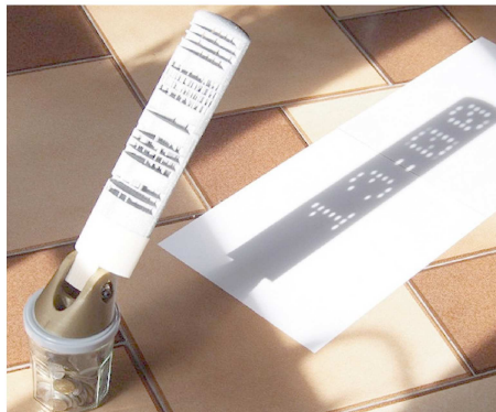
Digital sundial (3d-printed)
