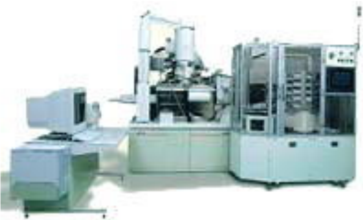
Example of an electron beam lithography equipment from JEOL
